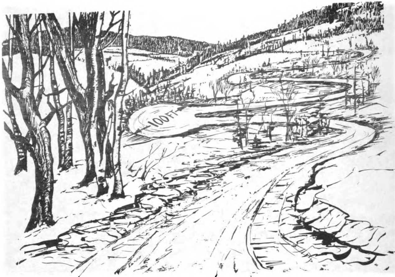
Figure 4-5. Development of switchbacks.
